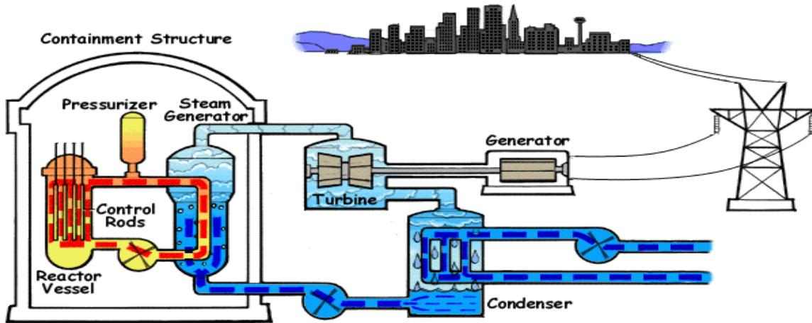
designs make use of two to six steam generators, each associated with a coolant loop.
