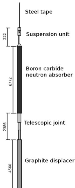
carbide itself sets exactly to the active area of the reactor. On top of the telescopic joint there is the boron carbide, which acts as a neutron absorber, slowing the reaction. This is affixed to a suspension unit, where a steel cable is connected. (*After the Chernobyl accident these steel wires were replaced with steel tapes.*) The suspension unit absorbs mechanical shocks from movement and prevents rods from twisting in their channels.
