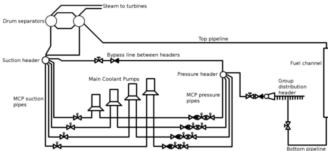
The drum separators are large cylinders with an outer diameter of 2.83 m and a length of 33.76 m. The length mentioned here is a modification done on the Ignalina Nuclear Power Plant; other plants use about 30 m long drum separators. The separators are
